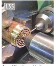
Cross drilling the combination brake valve.
