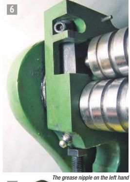
The grease nipple on the left hand side for the main shaft bearing and the top roll retainer.
