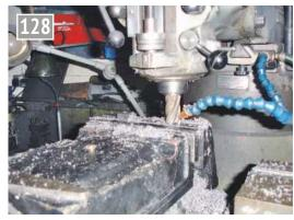
Machining the lifting links.
