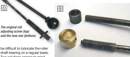
The 'pip' machined on the screw to stop the bearing rotating.
