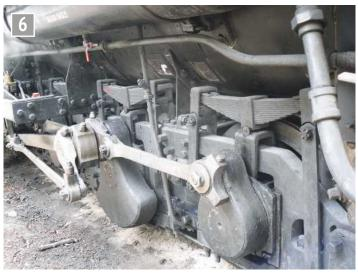
473 left hand side showing springs, frames and Y shaped end to the rear coupling rod.
