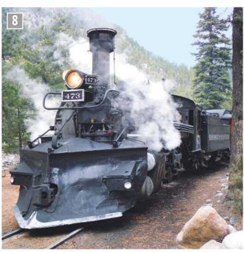
473 front end showing the snow plough and white painted points for applying pushing pole.
