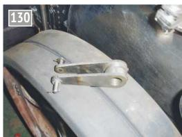
The completed lifting link levers.
