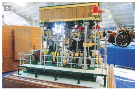
A typical triple expansion marine engine by Richard Simpson.
