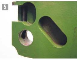
The main bearing with the roll retainer socket machined into it.
