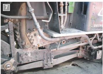
473 left hand rear truck assembly and bolted frame extension.
