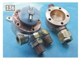
The fully functioning steam brake valve.
