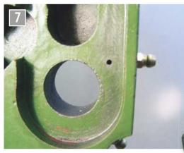
The grease nipples for the right-hand side showing the hole for greasing the gears.
