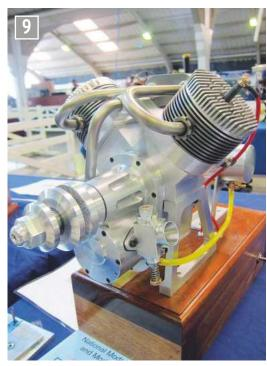
Tom Pasco's 30cc Vee twin supercharged sleeve valve two stroke engine.
