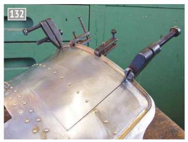
The cab roof and the addition of further rain strips.
