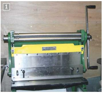
The three-in-one combination of shear, press brake and roll.
