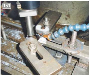
Machining a radius in the reversing lever.
