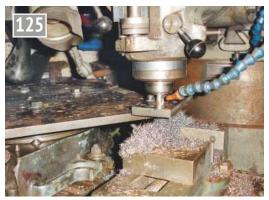
Cutting the slot in the expansion link.
