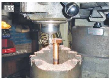
Milling the hexagon on the valve guide head.
