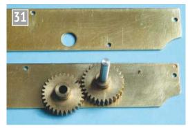
Using pointed steel rod to mark gear centres.
