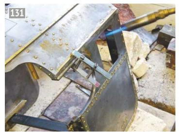
Soldering a rain strip into position; a tricky operation.
