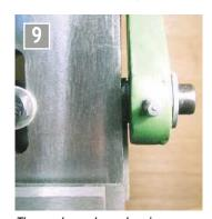
The crank arm lower bearing grease nipple.
