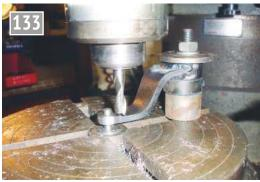
Profiling the lifting lever.
